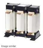
LINE REACTOR F. FC; PHASES:3; UN1(V):480; ITHMAX 1(A) / F1(HZ):560 /60; I LN (A):504; UK(%):4; LN(MH):0.0503; TA/ISO. CL:40 /H; IP00; CONNECTION:FLAT-TYPE TERMINAL; EN 61558-2-20 >UL/ CSA-RECOGNIZED< > REACTOR<
